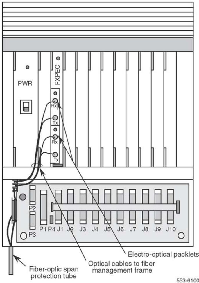
Figure 16: Link connections on the IPE cabinet
