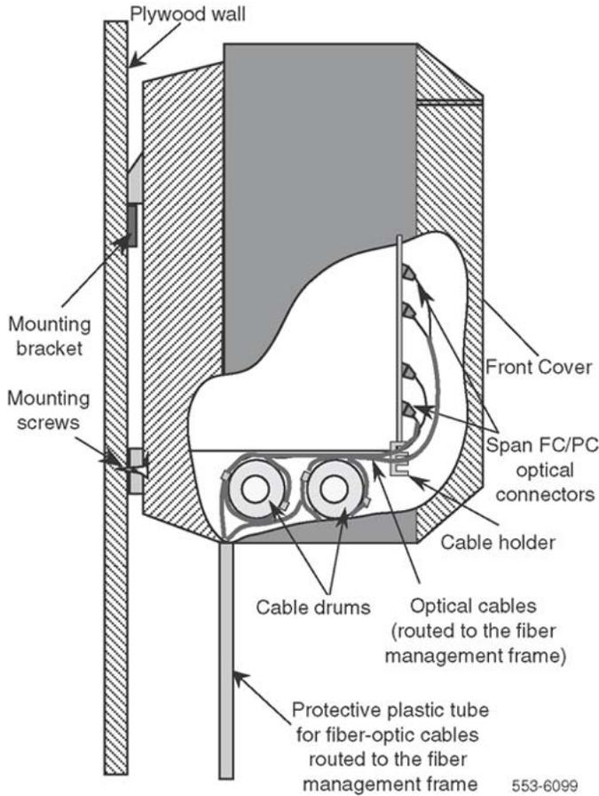
**Figure 15: Optical cable routing for the wall-mounted cabinet**
