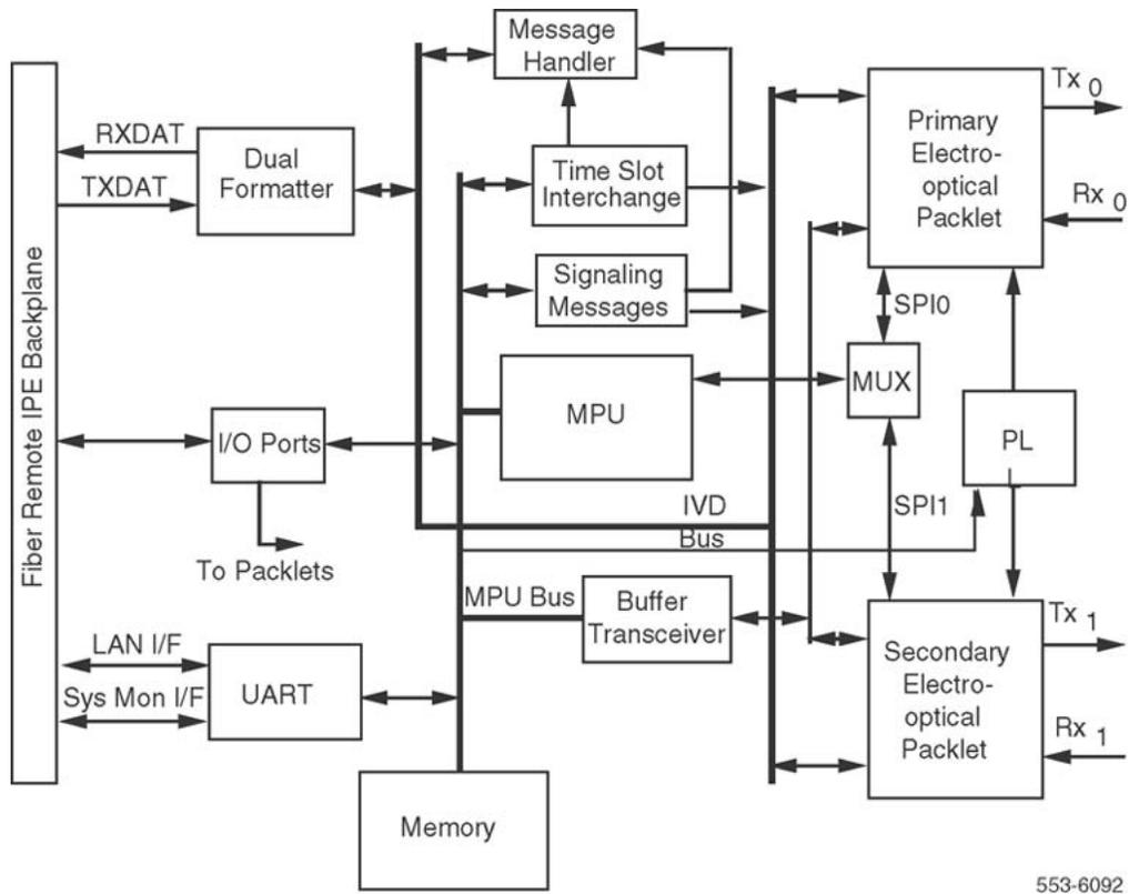
Figure 7: Fiber Peripheral Controller card functional block diagram
