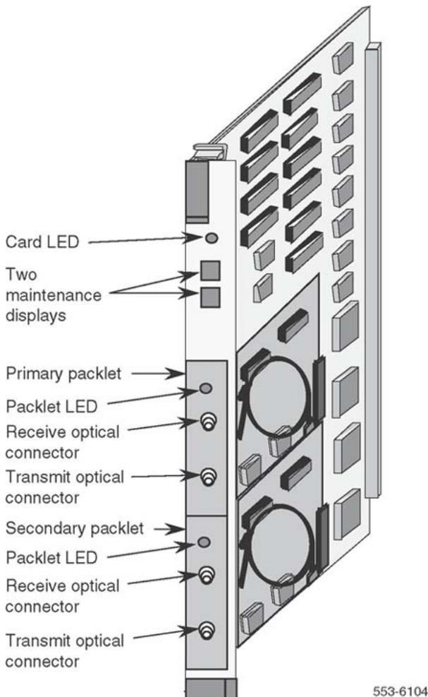
**Figure 20: Fiber Peripheral Controller card**
