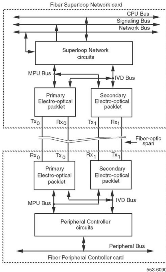
**Figure 5: Fiber Remote architecture**
