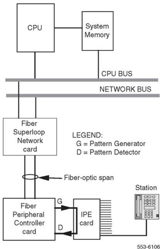
**Figure 22: Loopback path for XCON test 7**
