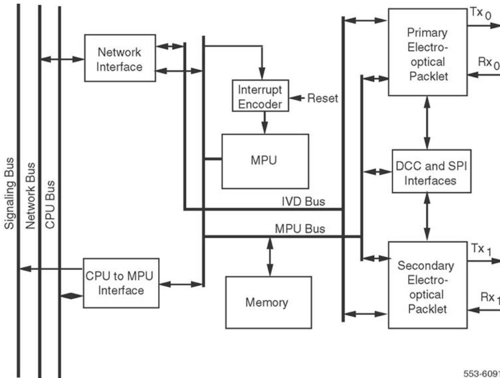
**Figure 6: Fiber Superloop Network card functional block diagram**
