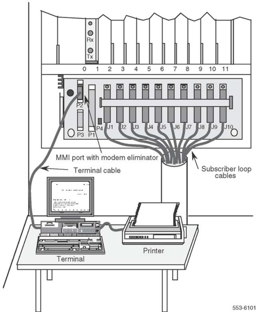
Figure 17: TTY and subscriber loop cable connections
