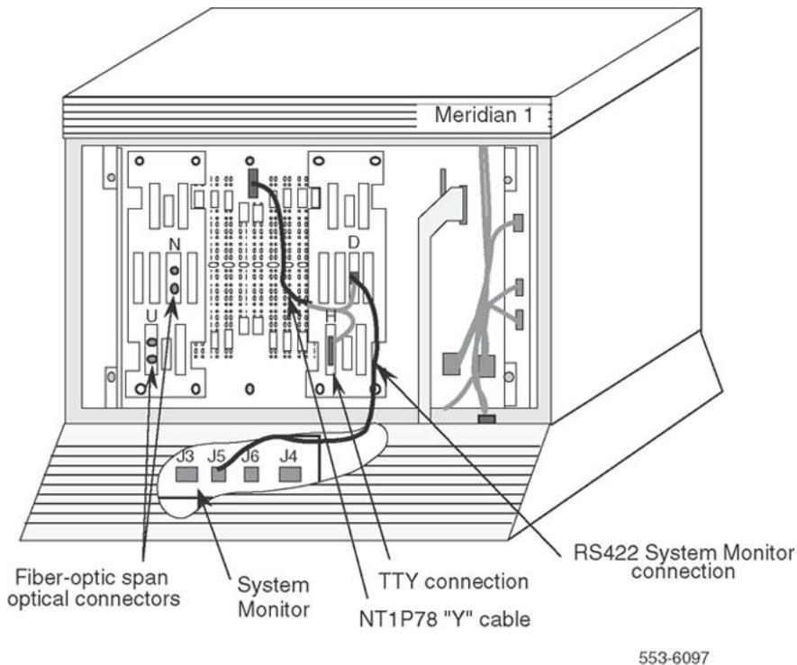
**Figure 13: System monitor and TTY cable connections**
