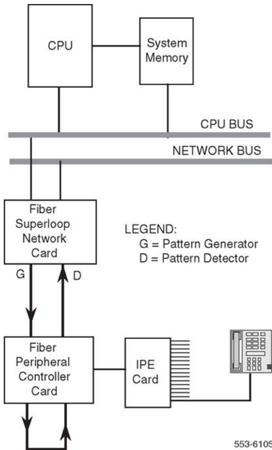
**Figure 21: Loopback path for XCON test 6**
