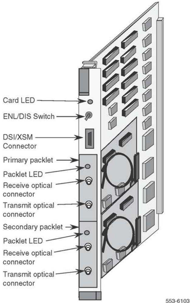
**Figure 19: Fiber Superloop Network card**
