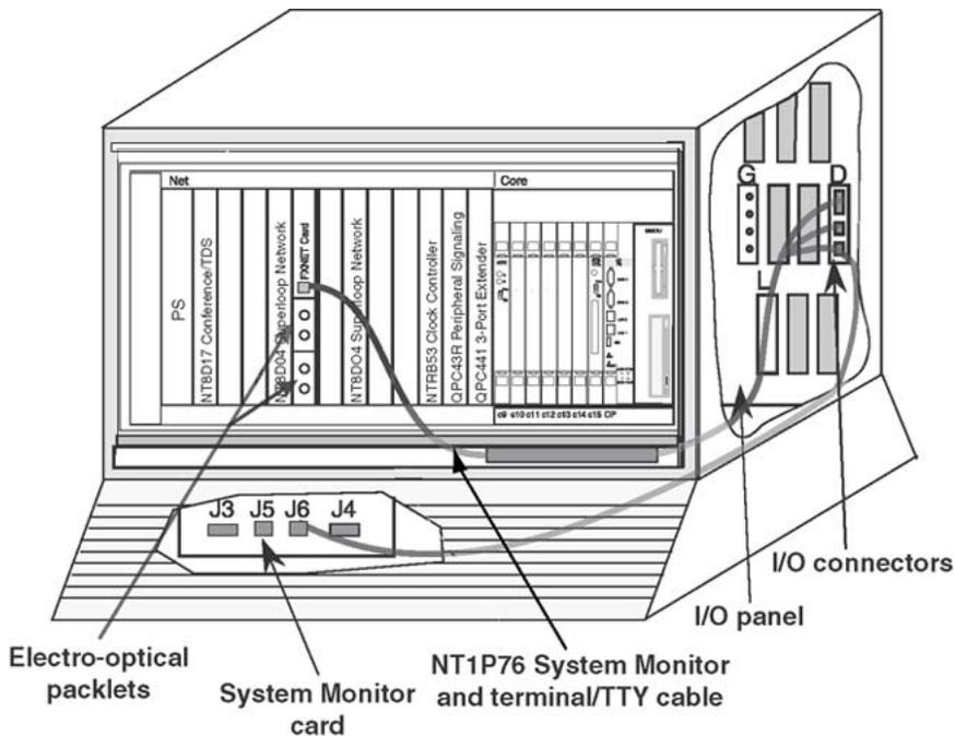
**Figure 10: System monitor and TTY cable connections**
