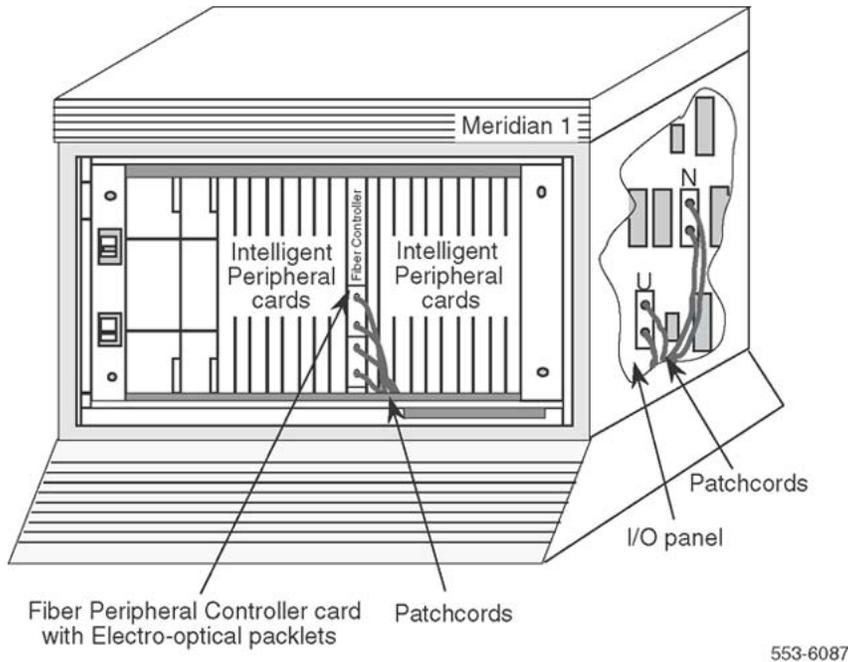
**Figure 2: Floor-standing Fiber Remote IPE column**
